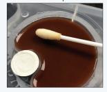
Inoculate the specimen by rolling the sample swab on the surface of the medium in a large "C" pattern for maximum transfer. For isolated colonies, cross-streak with the sterile inoculation
